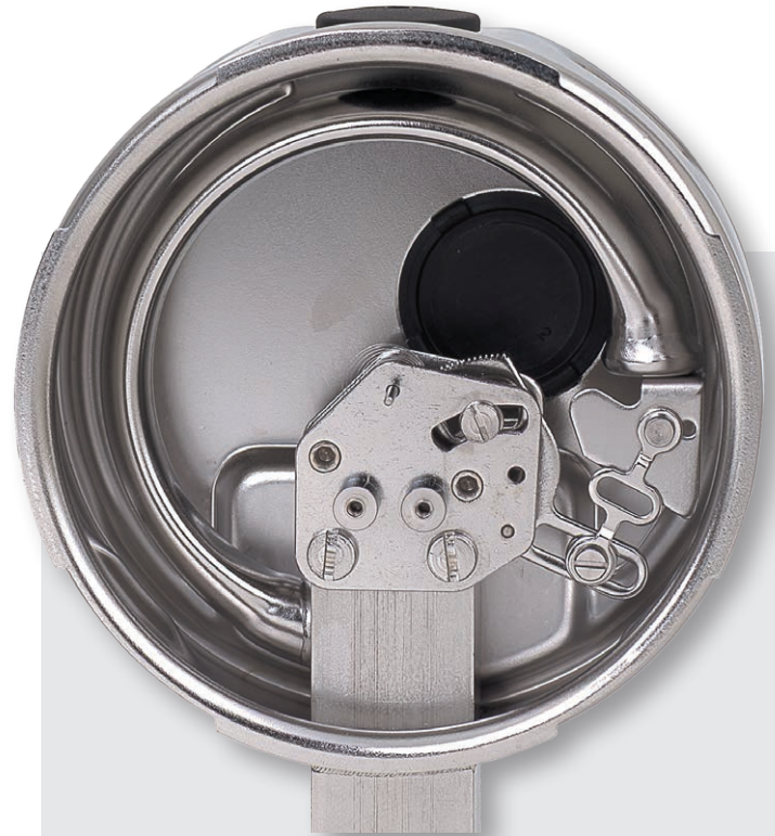
Internal workings of a mechanical pressure measuring instrument
